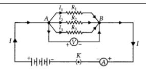
It is observed that the total current I, is equal to the sum of the separate currents through each branch of the combination.
