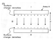
Electric field between the plates of capacitor
